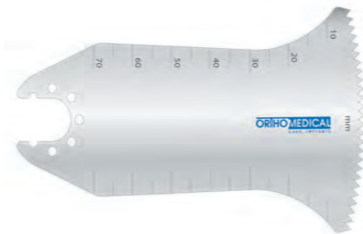
95-349.63VET Blade thickness 0.6mm / Cut thickness 0.8mm / Tooth pitch (TPI)1.9mm / Useable length 71mm / Blade width 50mm
